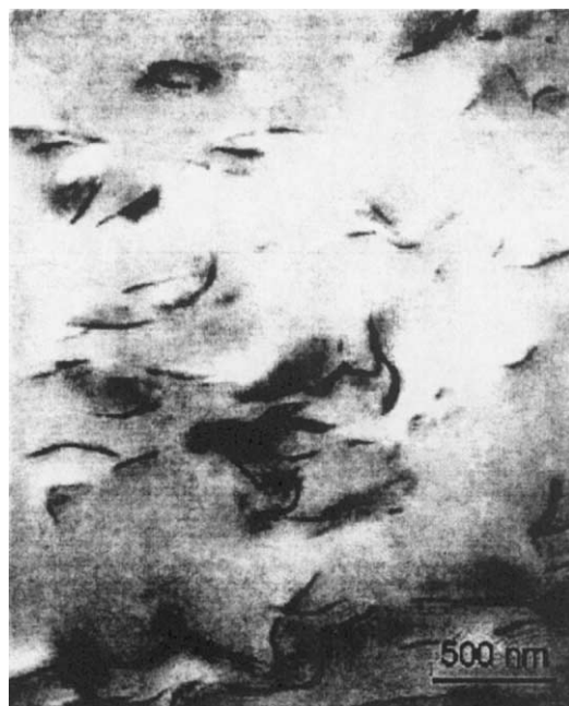
Fig. 5. TEM photo of 3% clay APB–BPDA films showing exfoliated clays.
